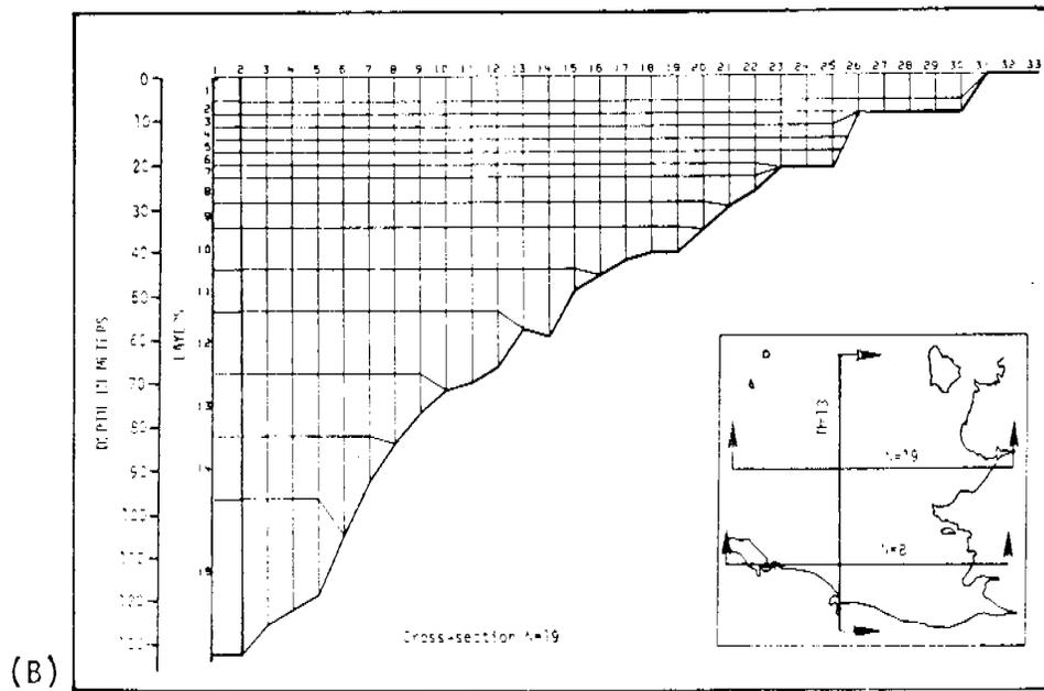
Fig. 4--Horizontal (A) and vertical (B) distribution of grid dimensions, showing the arrangement of layer thickness in the Bristol Bay model
