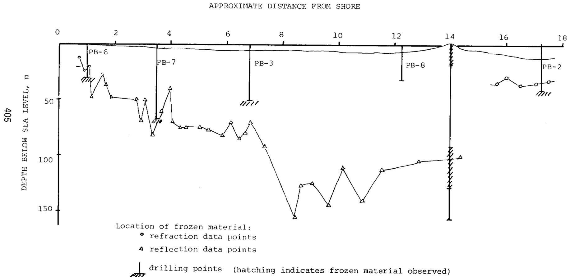
Figure 2 - Vertical section from new ARCO dock through Reindeer Island.
